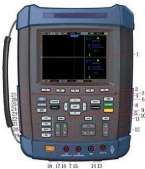
Multifunctional Partial Discharge Tester main tester front panel
