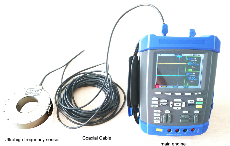
High frequency current transformer connection
