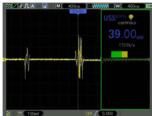
with discharge signals
