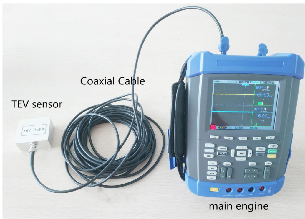
Composite TEV sensor wiring
