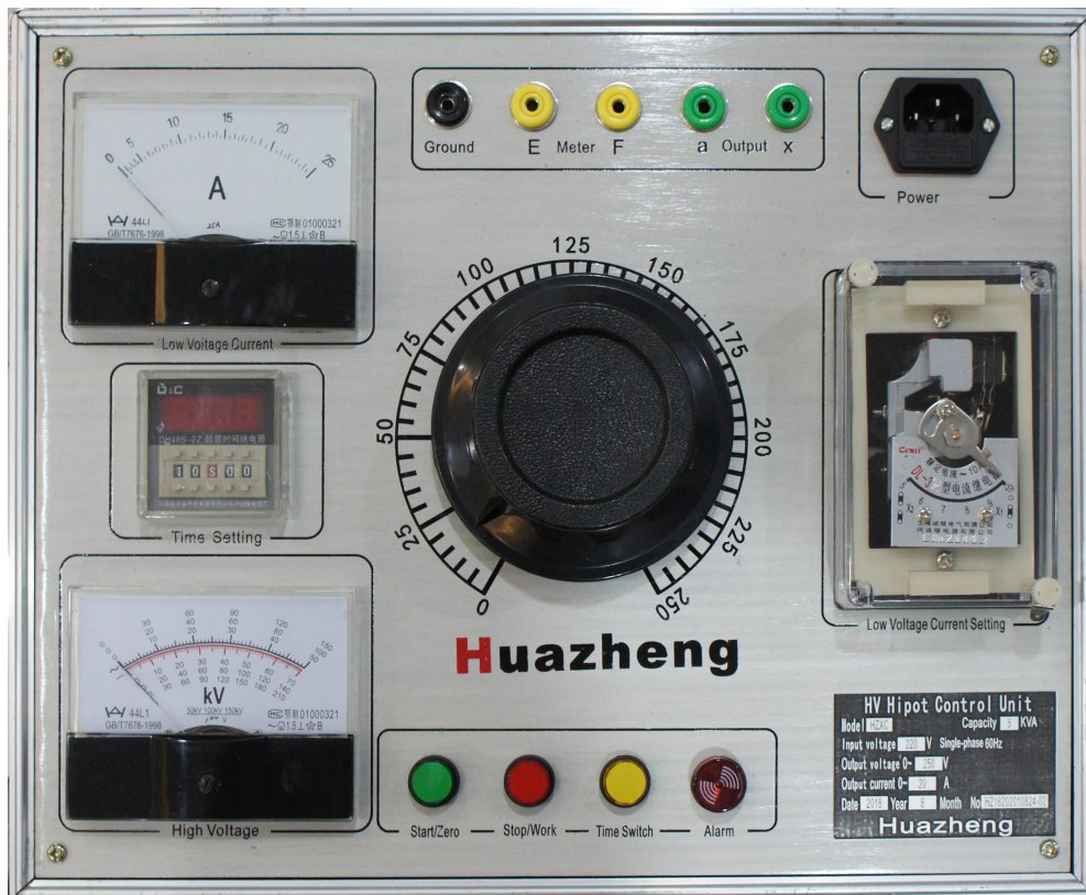
Figure 4 Panel of main control box
